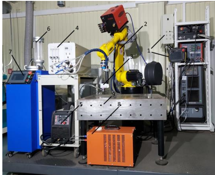
Fig.3. A robotic set of equipment for automatic 3D printing of small and medium-sized metal objects by microplasma deposition, limited by the reach of the robot arm up to 1400 mm: 1 – an intelligent control system with an integrated automatic monitoring system; 2 – movement mechanism (robot); 3 – microplasmatron; 4 – plasma module; 5 – power source; 6 – powder dispenser-feeder; 7 – powder feeder control unit; 8 – autonomous cooling unit; 9 – assembly and surfacing device, surfacing table.
