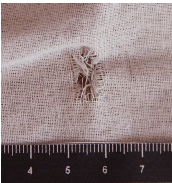
Fig. 6. Damage to cotton fabric caused by a shot from Fort 12R at a distance of 50 cm.
