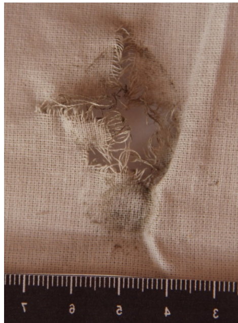
Fig. 1. Damage to cotton fabric when shot at close range with the AE790G1.
